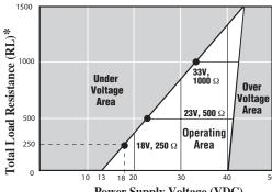
**Power Supply Voltage (VDC)** \*NOTE: Cable resistance effect included in RL.
